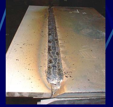
Three pass V-groove using constant volume fill
